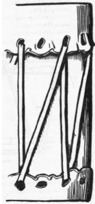
Fig. 9: Lacing in an N pattern.
